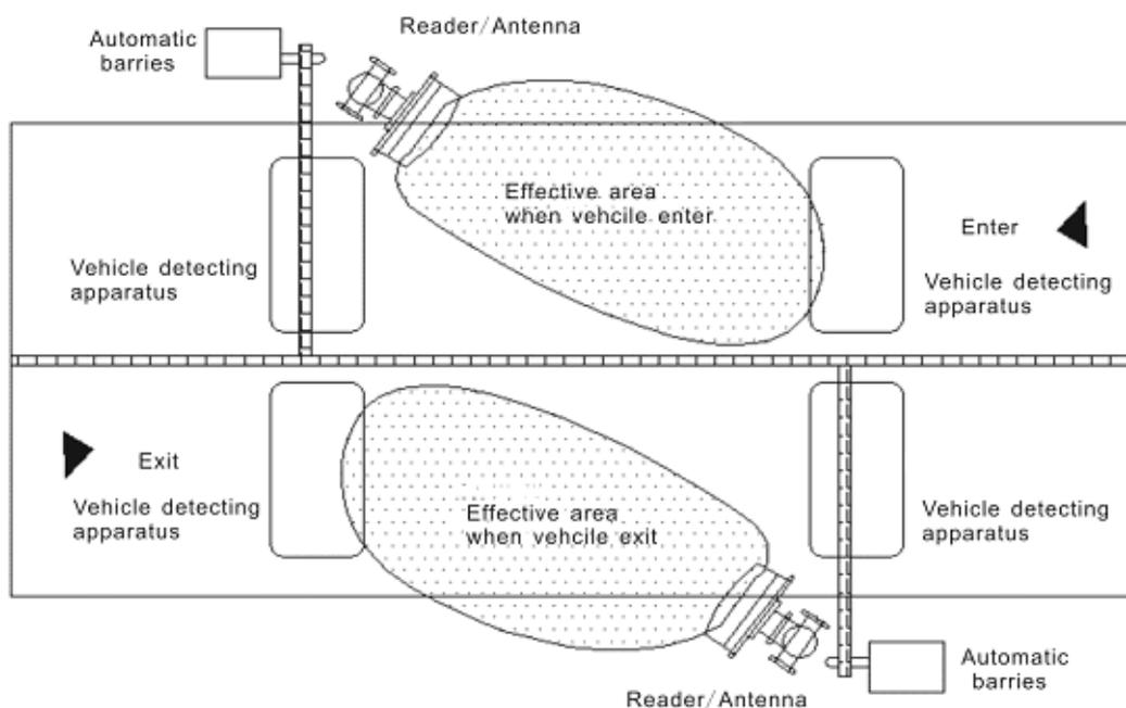
Figure 3 Installing method 1
