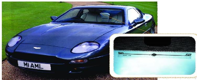
Figure 5 RFID tag mounted on the windshield
