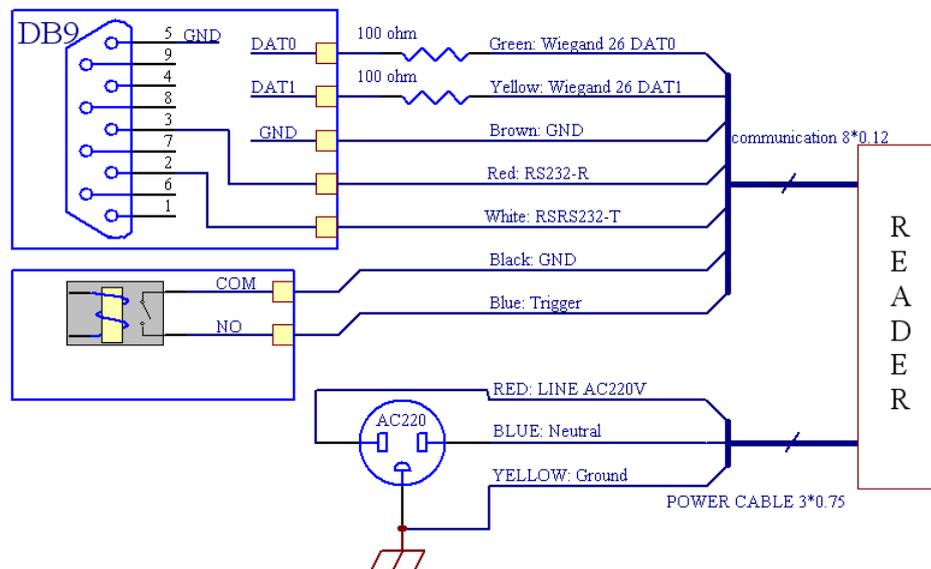
On AC 220V aerial socket, No. 1 is neutral, No. 2 is hot, and No. 3 is ground.
