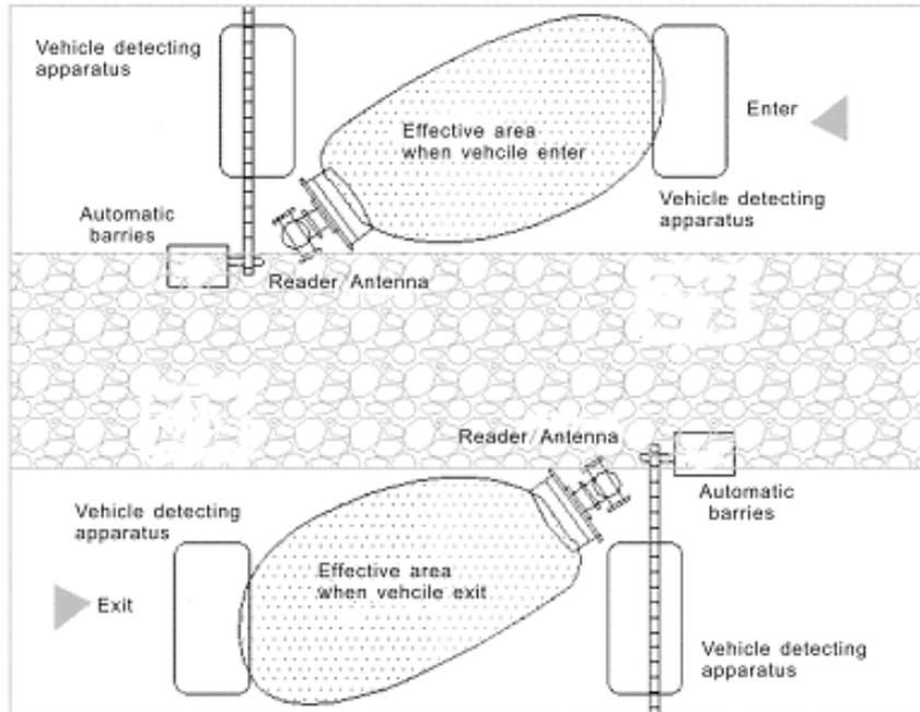
Figure 4 Installing method 2
